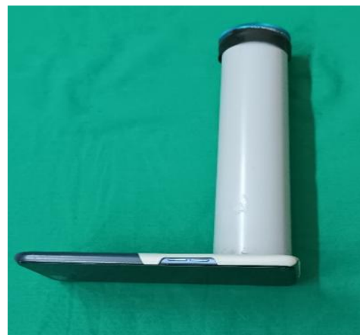
Fig.2 Adaptor with phone and 20D lens
