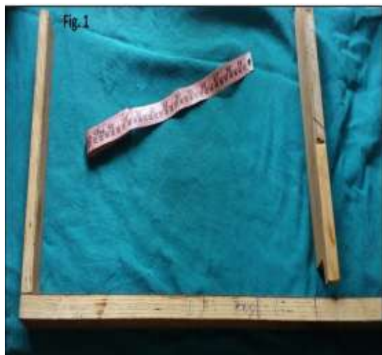
Fig.1: Photograph of the wooden frame used to measure the width of the bovine at the centre of X-ray beam exposure.
