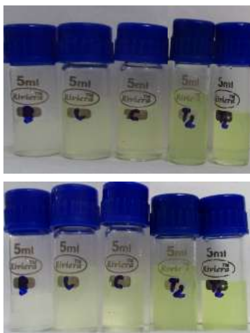
Fig. 1: FDA hydrolysis in control and treatment groups on 30th day of refrigeration storage (1st bottle=blank, next two bottles=control, last two bottles= treatment)
