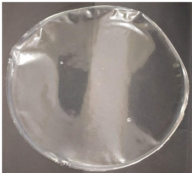
Figure 1: Edible packaging film (treated with 0.5% clove oil)
